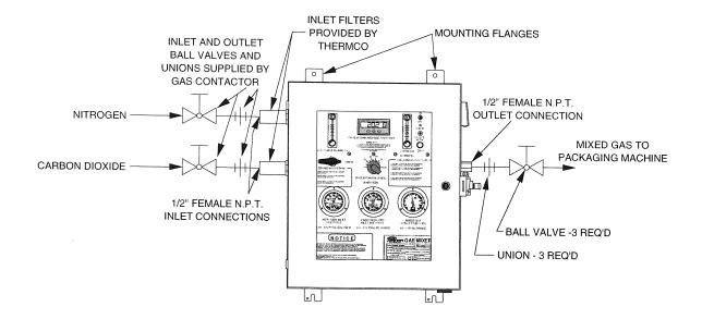
Mounting Location: Gas mixer should be mounted indoors; operating temperature range is 40°F to 104°F. Gas mixer enclosure is rated NEMA 4X; the gas mixer may be mounted in wet/washdown areas.
