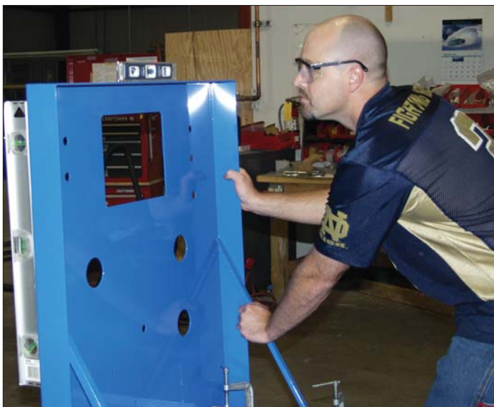
A panel is checked for squareness while being attached to a surge tank by Scott Hakes of the Prep & Shipping Departments.
