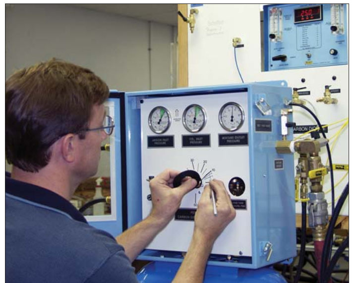
The scale of a Model 8500 gas mixer is applied by Steve Hixon, Gas Mixer Technician.
