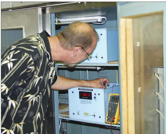
Dana Wooten, Gas Analyzer Technician, prepares an analyzer for temperature testing in the environmental chamber.
